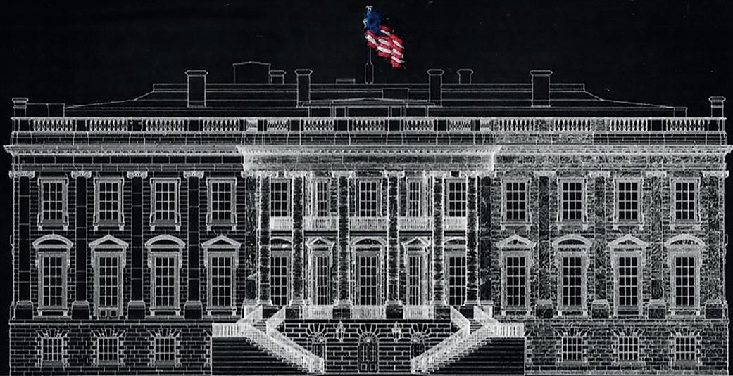
FULL ELEVATION ELEVATION SHOWING GRAN PATTERN OF AQUA SANDSTONE
